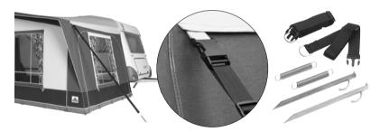
In order to prevent any serious damage from happening to the awning canvas it is important that you always use the straps in combination with the springs. For the correct use of the system, fix the peg at about 50 cm. distance from the side of the awning. The spring should then be fixed between the round shaped eye on the top of the peg and the oval shaped eye at the bottom of the strap. When tensioning the strap make sure that the spring is under medium tension.
