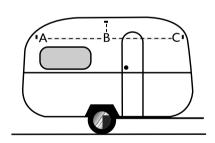
in the picture (above point B). The measurement between A-B and B-C should be equal. Screw the plastic eyes parallel approximately I cm. from the rail, so that the hooks on the frame can be attached without any obstruction. The possible two additional eyes should then be fixed between A-B and B-C.
